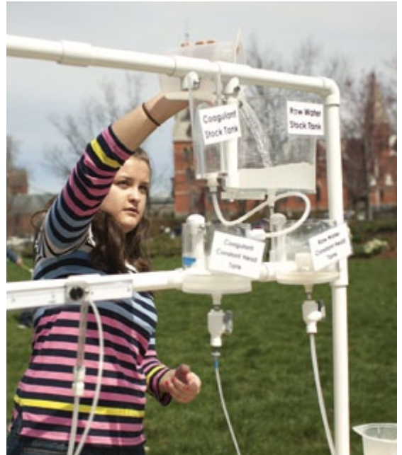
AguaClara Team Leader Julia Morris operates the program’s demonstration plant, which represents the processes used to treat water in AguaClara municipal-scale drinking water treatment plants.
